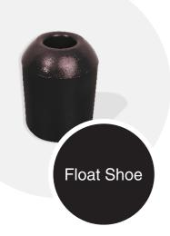
Pinnacle's PDC drillable integrated check valve in float shoe prevents fluids from entering casing as its being lowered into the hole. It also inhibits reverse flow or U-tubing of cement from annulus into the casing while allowing circulation down through the casing.
